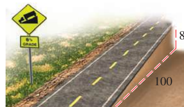
Grade of a road \text{Slope} = \frac{8}{100}
